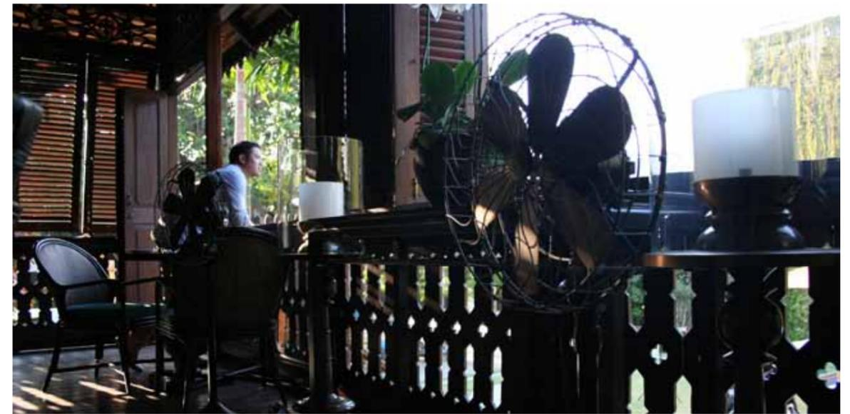
techniques used in the Idea House (Malaysia) were drawn from the traditional Malay Kampong houses that were built before the advent of electricity – and therefore air-conditioning. They were designed in a way that would maximise natural ventilation, such as high roofs that would allow the air to circulate, and open verandas surrounded by foliage that would cool the breeze as it passed through the house.
